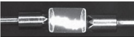
Standard Capacitor with Surface Arc-over
