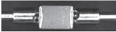
HVArc Guard® Capacitor with no Surface Arc-over
