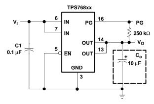
Figure 26. Typical Application Circuit (Fixed Versions)
