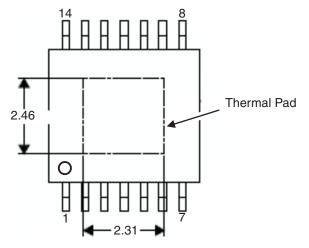
Figure 13. Thermal Pad Dimensions
