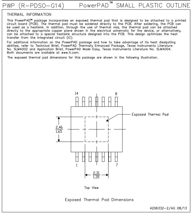
NOTE: A. All linear dimensions are in millimeters
