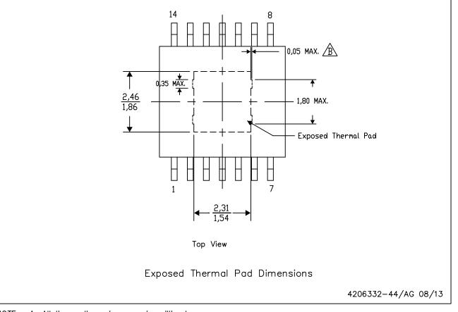
NOTE: A. All linear dimensions are in millimeters A. Exposed tie strap features may not be present.
