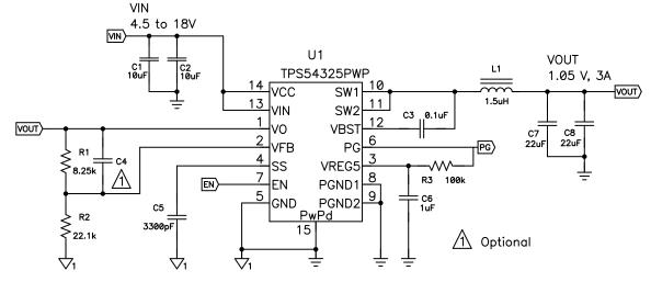
Figure 12. Schematic Diagram for this Design Example
