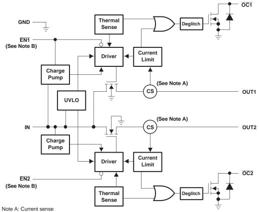
Note B: Active low  $(\overline{ENx})$  for TPS2062. Active high (ENx) for TPS2066.
