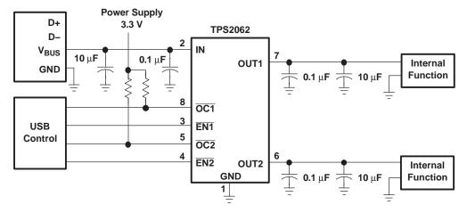
Figure 28. High-Power Bus-Powered Function
