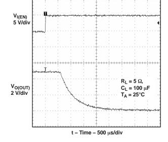
Figure 5. Turnoff Delay and Fall Time With 100-µF
