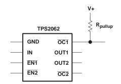
Figure 26. Typical Circuit for the OC Pin
