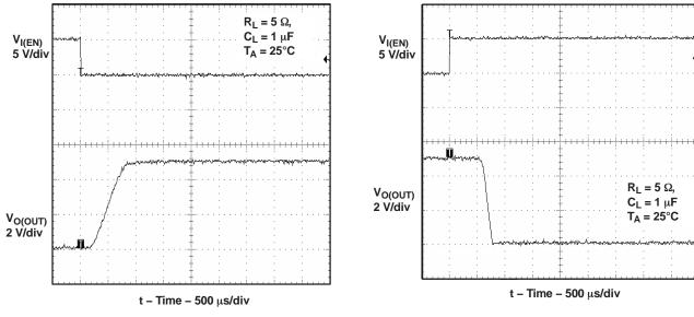
Figure 1. Test Circuit and Voltage Waveforms
