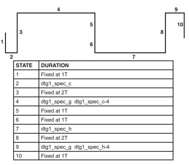
Figure 4-32. SDTV Line Type NEQ\_BSP
