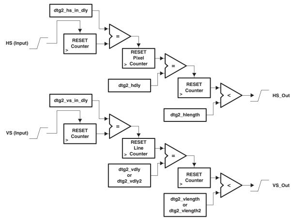
Figure 4-15. THS8200 DTG VS/HS Output Generation
