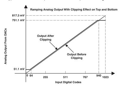
Figure 4-5. Effect of Clipping on Analog Output
