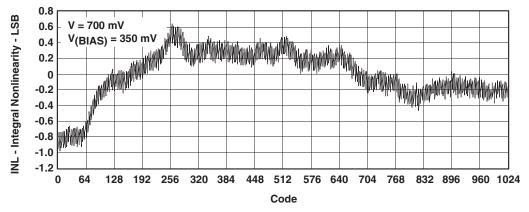
Figure 7-7. Integral Nonlinearity vs Code
