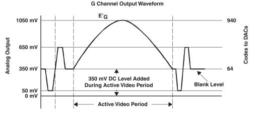
Figure 4-41. G-Channel Output Waveform
