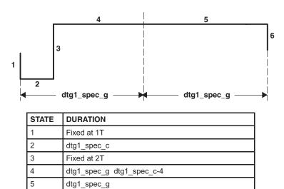
Figure 4-34. SDTV Line Type FULL\_NEQ
