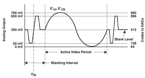
Figure 4-46. Analog Output of Cr and Cb Channels With Sync Insertion
