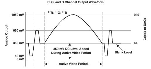
Figure 4-43. R-, G-, and B-Channel Output Waveform
