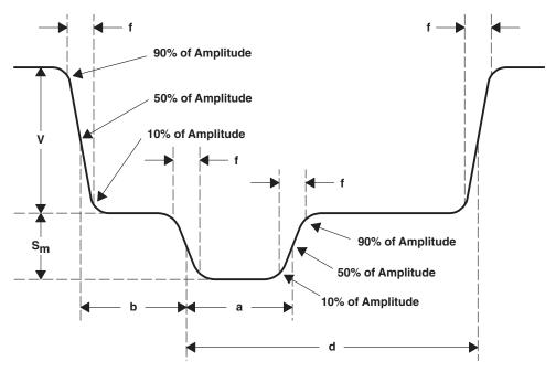
Figure 4-26. Horizontal Synchronization Signal Waveform
