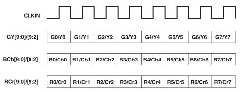
Figure 4-1. 24-/30-Bit RGB or YCbCr Data Format
