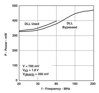
Figure 7-2. Power vs Frequency
