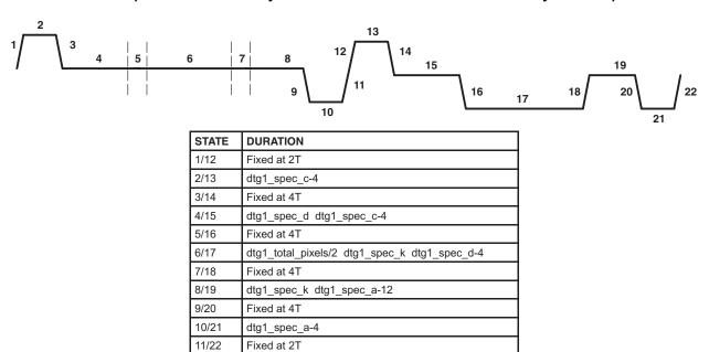
Figure 4-22. HDTV Line Type NTSP\_BTSP
