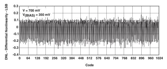
Figure 7-8. Differential Nonlinearity vs Code
