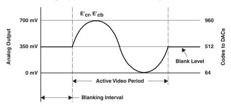
Figure 4-45. Analog Output of Cr and Cb Channels Without Sync Insertion
