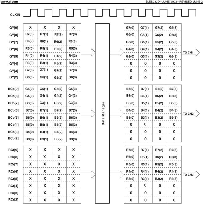
Figure 4-4. 15-Bit RGB 4:4:4 Data Format
