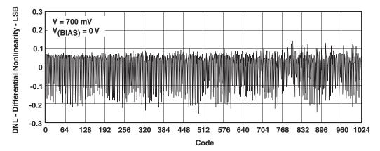
Figure 7-6. Differential Nonlinearity vs Code
