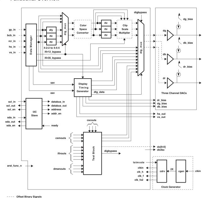
Figure 3-1. Functional Block Diagram
