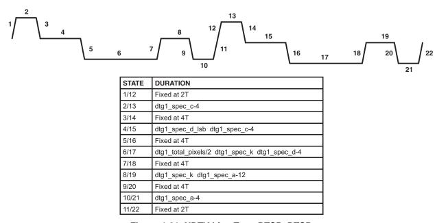
Figure 4-21. HDTV Line Type BTSP\_BTSP
