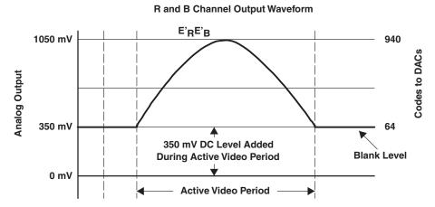
Figure 4-42. R- and B-Channel Output Waveform
