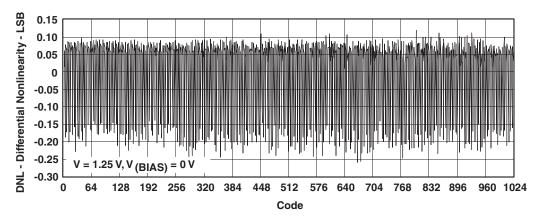
Figure 7-10. Differential Nonlinearity vs Code
