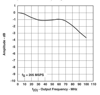
Figure 7-11. Amplitude vs Output Frequency
