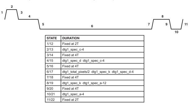
Figure 4-24. HDTV Line Type FULL\_BTSP
