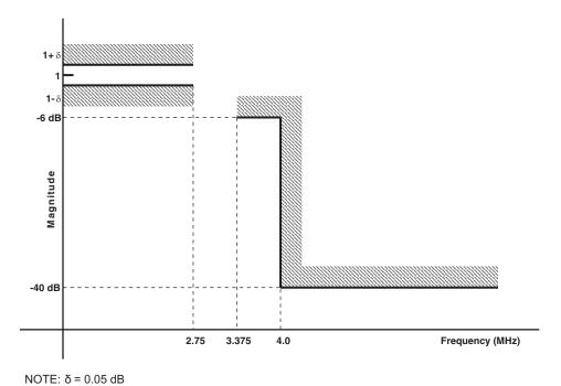
Figure 4-11. Cb and Cr Filter Requirements Based on ITU-R.BT601
