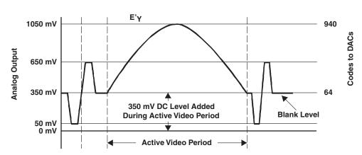
Figure 4-44. Y-Channel Output Waveform
