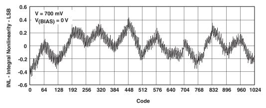
Figure 7-5. Integral Nonlinearity vs Code
