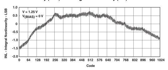
Figure 7-9. Integral Nonlinearity vs Code
