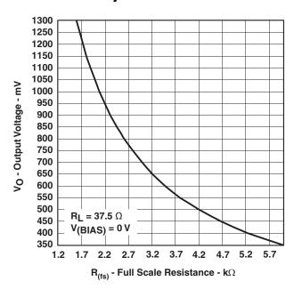
Figure 7-12. Output Voltage vs Full-Scale Resistance
