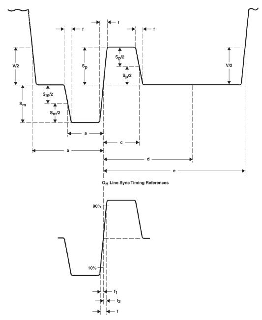
Figure 4-16. Tri-Level Line-Synchronizing Signal Waveform
