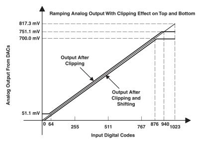
Figure 4-6. Effect of Shifting on Clipped Analog Output
