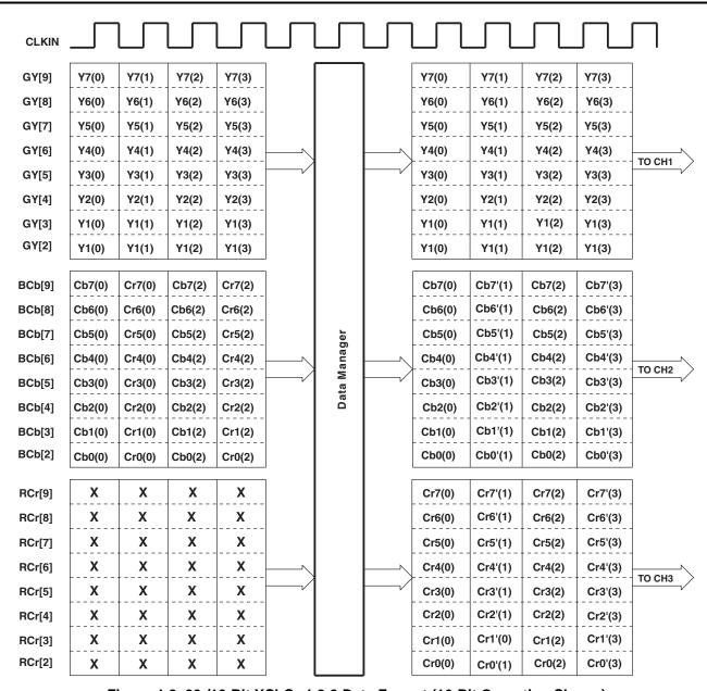
Figure 4-2. 20-/16-Bit YCbCr 4:2:2 Data Format (16-Bit Operation Shown)
