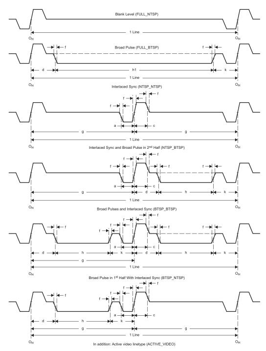
Figure 4-17. THS8200 VBI Line Types in HDTV Mode
