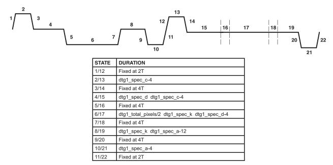
Figure 4-23. HDTV Line Type BTSP\_NTSP
