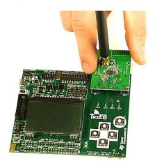
Insert a CC1200EM board into the TrxEB as shown above. Connect the antenna to the SMA connector on the EM.
