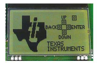
Turn on power with the Main Power switch. You should now see the Texas Instruments logo and a short description of the buttons on the LCD. Pushing any of the five buttons on the board will take you to the main menu.
