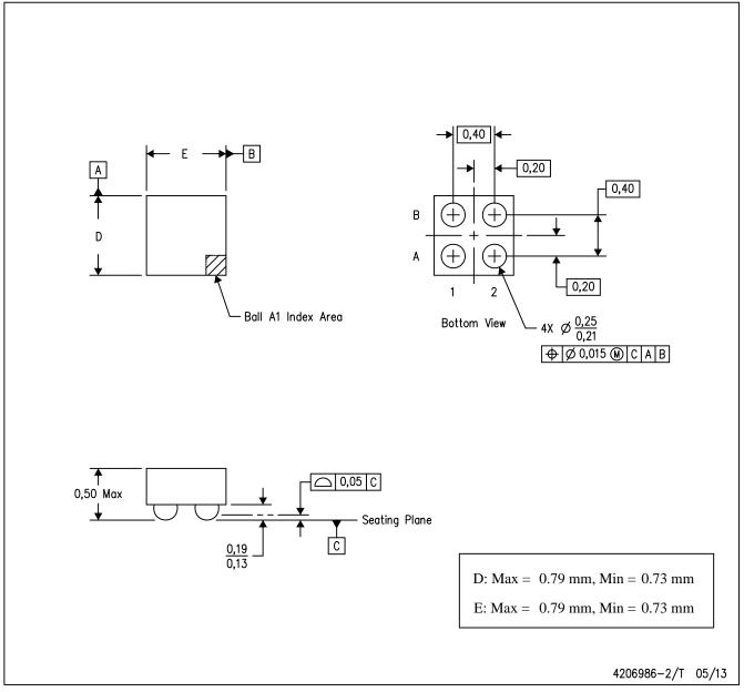
NOTES: A. All linear dimensions are in millimeters. Dimensioning and tolerancing per ASME Y14.5M-1994.
