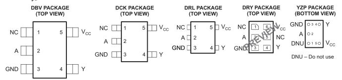
NC – No internal connection See mechanical drawings for dimensions.
