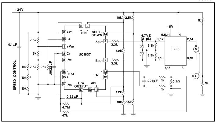
Figure 7. Bi-Directional Motor Drive with Speed Control Power-Amplifier
