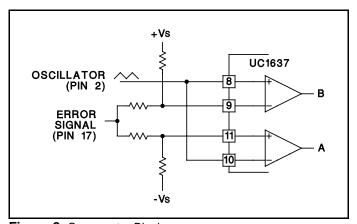
Figure 2. Comparator Biasing
