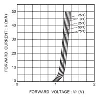
Fig.2 Forward current vs. forward voltage
