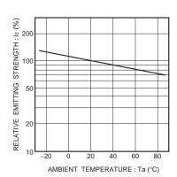
Fig.5 Relative emitting strength vs.ambient temperature
