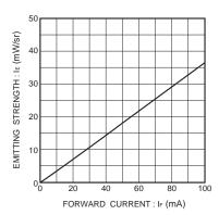
Fig.4 Emitting strength vs. forward current
