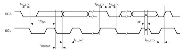
Figure 10. I2C Mode Timing
