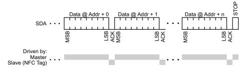
Figure 4. I2C Write Access
