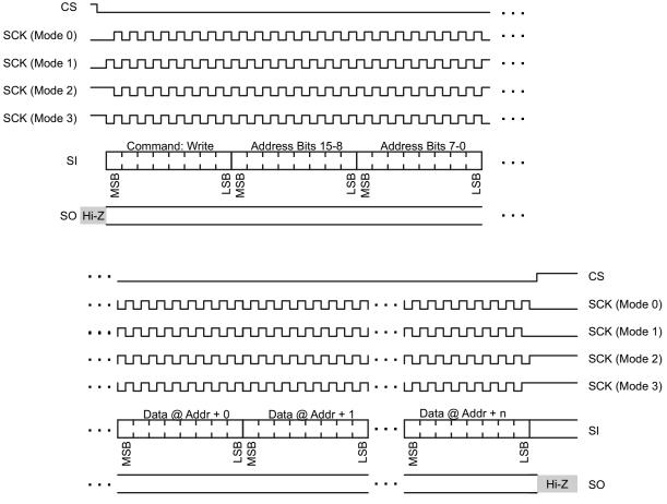
Figure 6. SPI Write Access
