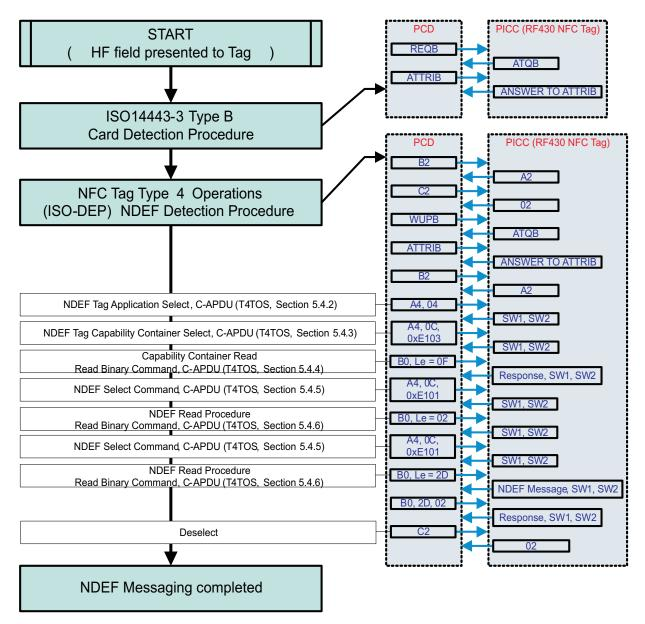
Figure 8. Command and Response Exchange Flow
