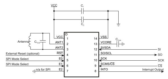
Figure 3. Example Application Diagram (SPI Operation)
