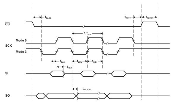
Figure 11. SPI Mode Timing
