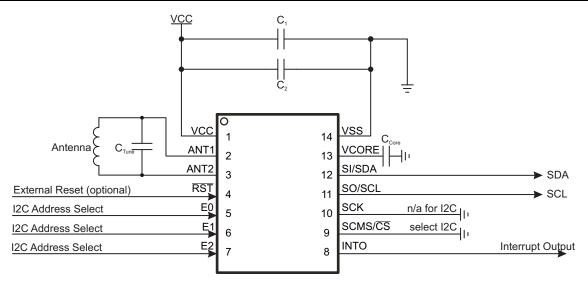
Figure 2. Example Application Diagram (I2C Operation)
