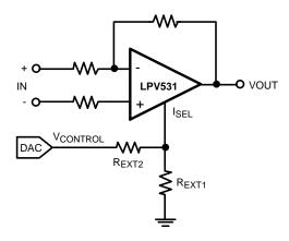
Figure 38. DAC Controlled Power Mode Configurations
