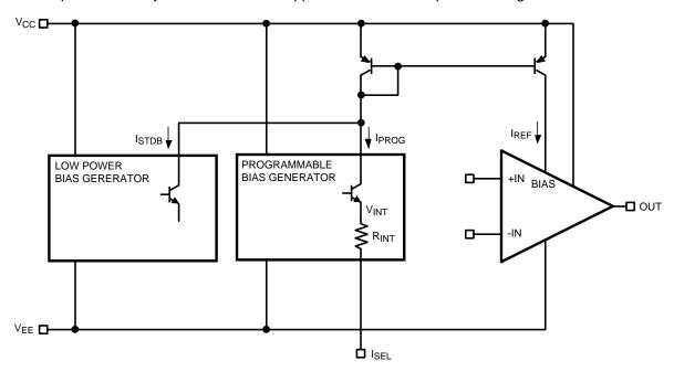
Figure 35. Simplified Schematic
