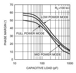
Figure 41. Phase Margin vs. Capacitive Load
