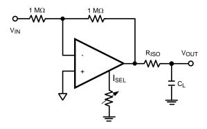
Figure 42. Compensation by Isolation Resistor
