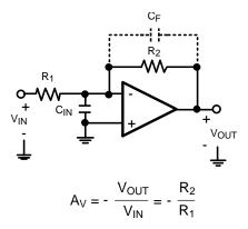
Figure 43. Inverting Amplifier
