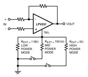
Figure 37. Power Modes Set by Resistors and Switches
