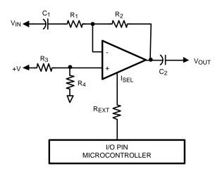
Figure 39. Inverting AC Coupled Application
