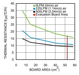
Figure 54. Package Thermal Resistance θ<sub>JA</sub> 4 Layer Printed Circuit Board with 1oz Copper
