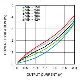
Figure 53. Power Dissipation  $V_{OUT} = 12V T_{AMB} = 85^{\circ}C$
