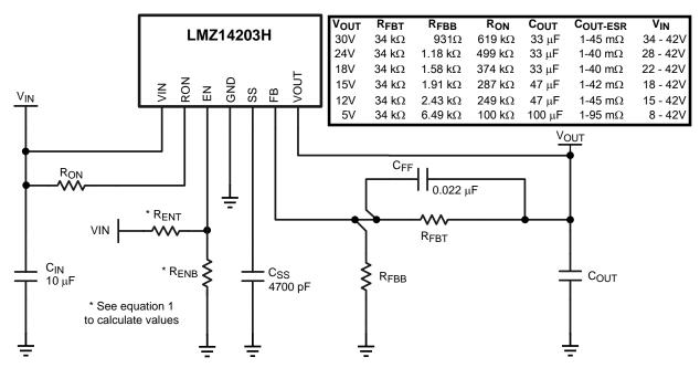
Figure 5. Simplified Application Schematic
