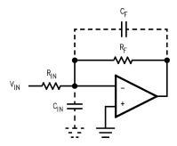
Figure 39. Cancelling the Effect of Input Capacitance
