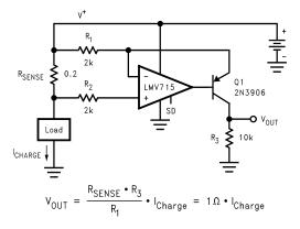
Figure 1. High Side Current Sensing
