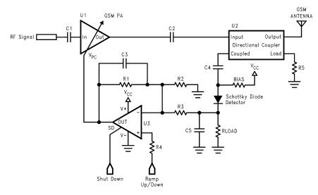
Figure 44. Typical of GSM P.A. Control Loop
