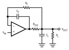
Figure 41. Indirectly Driving A Capacitive A Load with DC Accuracy
