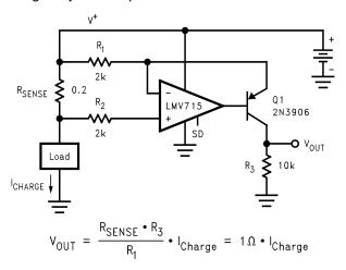
Figure 43. High Side Current Sensing
