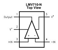
Figure 46. 5-Pin SOT-23 Package See Package Number DBV0005A
