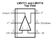
Figure 47. 6-Pin SOT-23 Package See Package Number DBV0006A
