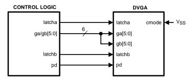
Figure 34. Parallel Mode Connection Using Latch Pins to Mulitplex Digital Data
