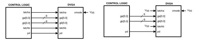
Figure 32. Parallel Mode Connection for Fastest Response
