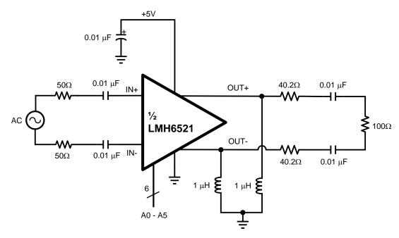
Figure 27. Basic Operating Connection
