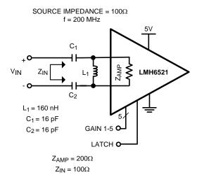
Figure 29. Differential 200Ω LC Conversion Circuit
