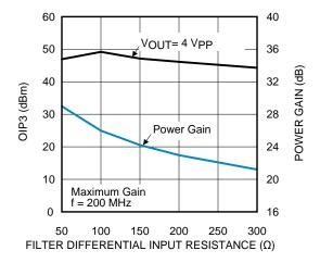
Figure 31. OIP3 vs Amplifier Load Resistance
