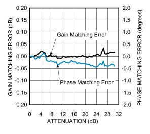
Figure 2. Channel Matching Error (Ch A - Ch B)
