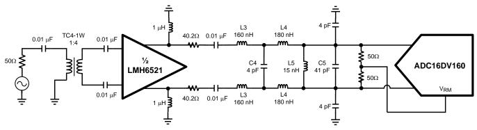
Center Frequency is 192MHz with a 20MHz Bandwidth. Designed for  $200\Omega$  Impedance.
