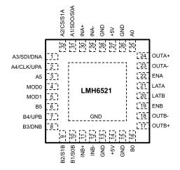
Figure 3. 32-Pin WQFN Package-Top View
