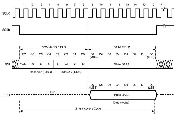
Figure 35. Serial Interface Protocol (SPI compatible)
