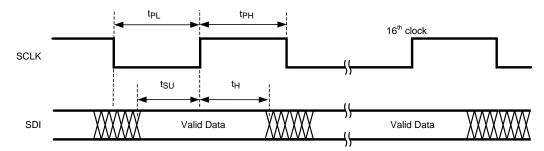
Figure 38. Write Timing, Data Written to SDI Pin
