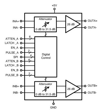
Figure 28. LMH6521 Block Diagram
