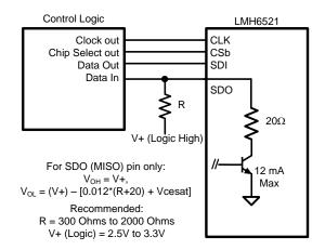
Figure 36. Serial Mode 4-wire Connection
