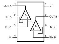
Figure 2. 8-Pin SOIC (Top View)
