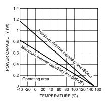
Figure 52. Power Capability vs. Temperature
