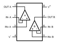
Figure 1. 8-Pin VSSOP (Top View)
