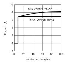
Figure 23. Transient Response to 7 Amp Step Current
