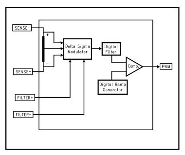
Figure 22. Functional Block Diagram of LM3812 and LM3813
