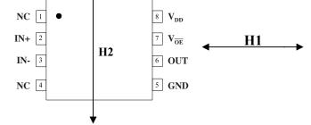
Regardless of orientation, driving the coil differentially improves magnetic immunity. This is because the logic high state is driven by an applied field instead of zero field, as is the case with single-ended operation. The higher the coil current, the higher the internal field, and the higher the immunity to external fields. Optimal magnetic immunity is achieved by adding the boost capacitor.
