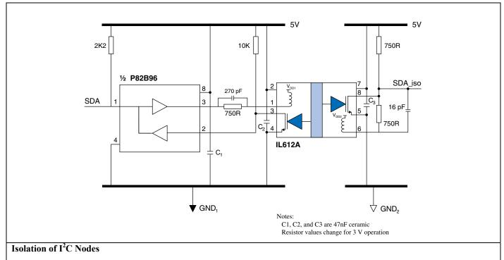
This circuit provides bidirectional isolation of I<sup>2</sup>C bus signals with no restrictions on data rate and none of the I<sup>2</sup>C bus latch-up problems common with other isolation circuits. The SCL section is similar as shown in the schematic using the other half of the P82B96.
