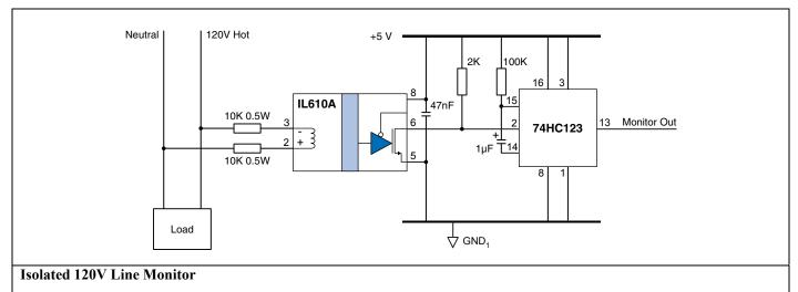
The wide input voltage range of IL600 Isolators allows connection to line voltage through current-limiting resistors. Unlike optocouplers, input voltage can reverse without damaging the inputs. In this illustrative circuit, "Monitor Out" goes low when line voltage drops significantly. The 74HC123 monostable converts the 60 Hz isolator output to a monitor signal.
