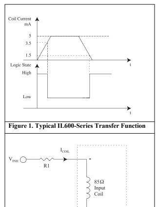
**Figure 2. Limiting Resistor Calculation**
