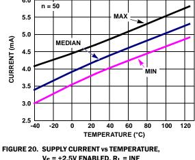
$V_S = \pm 2.5V$  ENABLED,  $R_L = INF$
