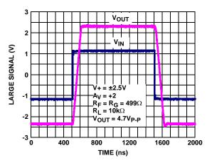
FIGURE 19. LARGE SIGNAL (4.7V) STEP RESPONSE
