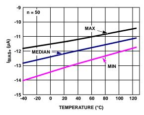
FIGURE 22.  $I_{BIAS+}$  vs TEMPERATURE  $V_S = \pm 2.5V$
