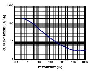
FIGURE 15. INPUT REFERRED NOISE CURRENT vs FREQUENCY
