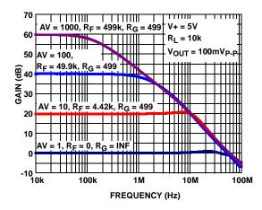
FIGURE 4. FREQUENCY RESPONSE vs CLOSED LOOP GAIN
