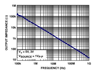
FIGURE 6. DISABLED OUTPUT IMPEDANCE vs FREQUENCY
