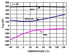
FIGURE 21.  $V_{OS}$  vs TEMPERATURE  $V_S = \pm 2.5V$
