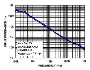
FIGURE 5. INPUT IMPEDANCE vs FREQUENCY
