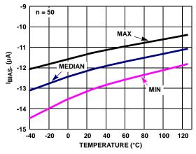
FIGURE 23.  $I_{BIAS}$  vs TEMPERATURE  $V_S = \pm 2.5V$
