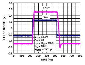
FIGURE 18. LARGE SIGNAL (1V) STEP RESPONSE
