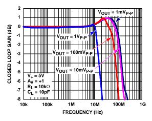
FIGURE 3. -3dB BANDWIDTH vs Vout
