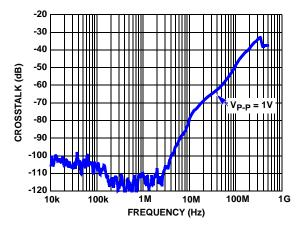
FIGURE 11. CHANNEL-TO-CHANNEL CROSSTALK vs FREQUENCY
