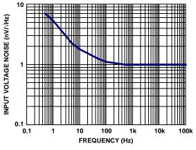
FIGURE 14. INPUT REFERRED NOISE VOLTAGE vs FREQUENCY
