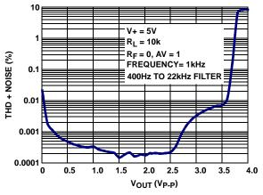
FIGURE 13. THD+N @ 1kHz vs  $V_{OUT}$
