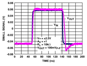
FIGURE 17. SMALL SIGNAL STEP RESPONSE
