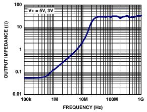
FIGURE 7. ENABLED OUTPUT IMPEDANCE vs FREQUENCY
