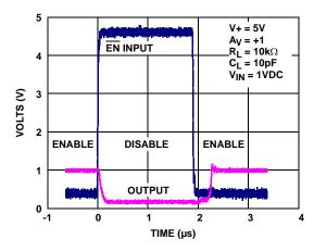
FIGURE 16. ENABLE/DISABLE TIMING
