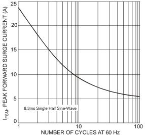
Fig. 4 Maximum Non-Repetitive Peak Forward Surge Current
