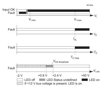
Fig. 12 Display status of LEDs
