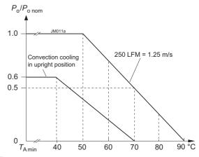
Fig. 4a Output power versus temperature T<sub>A</sub> at V<sub>inom</sub> (CPD/ CPA200)
