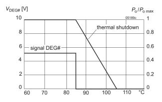
Fig. 9 Degrade signal  $V_{\text{DEG\#}}$  versus case temperature  $T_{\text{C}}$
