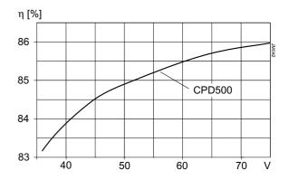
Fig. 2b CPD500 Series: Efficiency versus input voltage
