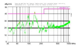
Fig. 14b CPA250-4530: Typical disturbance voltage at line input according to EN 55011/22, measured at V<sub>i nom</sub> and P<sub>o nom</sub>.
