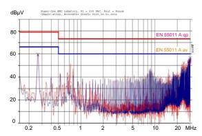
Fig. 14a CPA250-4530: Typical disturbance voltage at line input according to EN 55011/22, measured at V<sub>i nom</sub> and P<sub>o nom</sub>.
