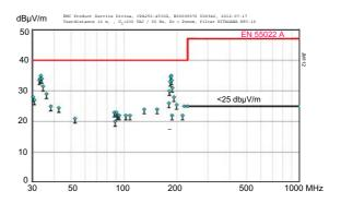
Fig. 14c CPA250-4530 with a core across the input lines. Radiated emissions EN 55011/22, measured at  $V_{\rm i\ nom}$  and  $P_{\rm o\ nom}$ .
