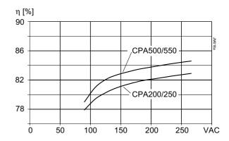
Fig. 2a CPA Series: Efficiency versus input voltage
