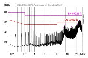
Fig. 13 CPD200/250: Typical disturbance voltage (peak) at line input according to EN 55022, measured at  $V_{\rm i\,nom}$  and  $P_{\rm o\,nom}$ .
