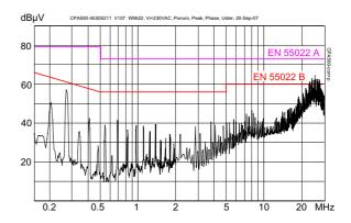
Fig. 15 CPA500-4530: Typical disturbance voltage (peak) at line input accord. to EN 55011/22, measured at V<sub>i nom</sub> and P<sub>o nom</sub>
