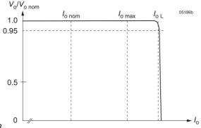
Fig. 3 Typical output characteristic Vo versus Io
