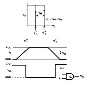
FIGURE 3. HYSTERESIS DEFINITION, CHARACTERISTIC, AND TEST SET-UP
