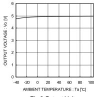
Fig.8 Output Voltage Temperature Characteristics
