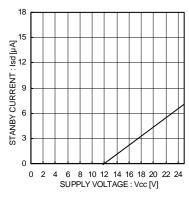
Fig.2 Shut Down Current
