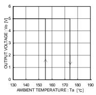
Fig.12 Thermal Shutdown Circuit Characteristics
