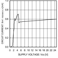
Fig.1 Circuit Current (IFEEDBACK\_R≒75µA)
