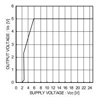
Fig.4 Line Regulation (Io=1000mA)
