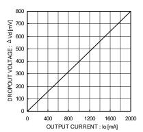
Fig.6 Dropout Voltage (Vcc=4.75V)
