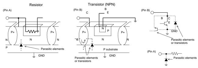
Example of Simple Monolithic IC Architecture
