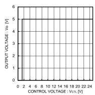
Fig.11 CTL Voltage vs Output Voltage
