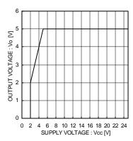
Fig.3 Line Regulation (Io=0mA)
