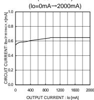
Fig.9 Circuit Current (IFEEDBACK\_R≒75µA)
