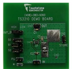
Figure 1. TS3310 Demo Board (Top View)
