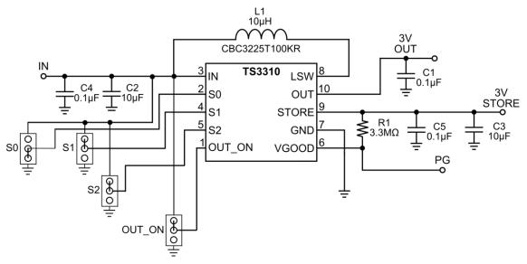
Figure 3. TS3310 Demo Board Circuit
