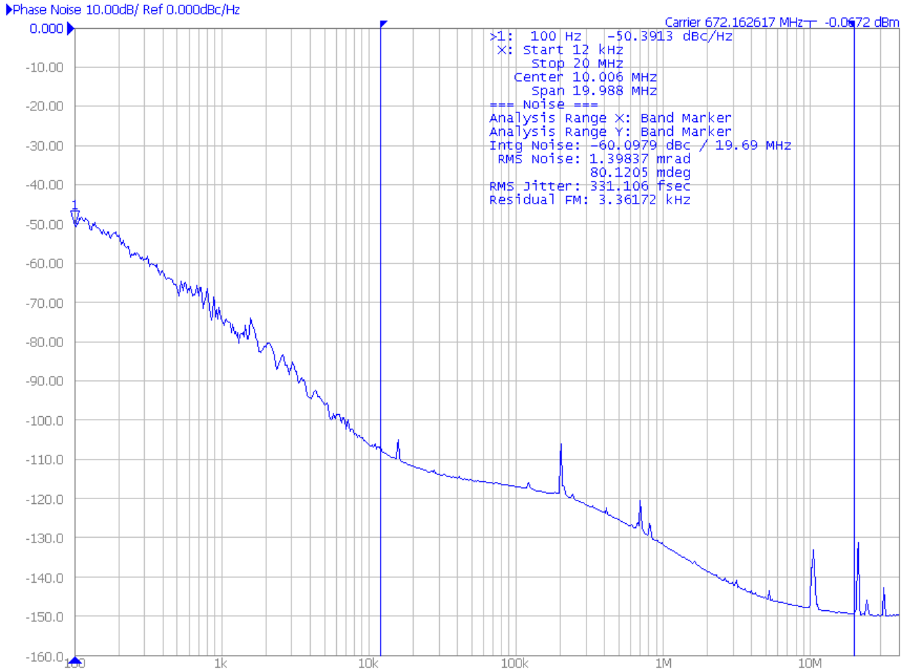
Figure 73. 622.08 MHz In; 672.16 MHz Out; Loop BW = 6.9 kHz
