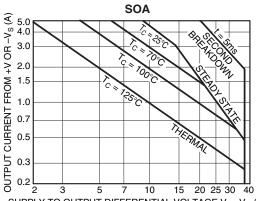
SUPPLY TO OUTPUT DIFFERENTIAL VOLTAGE V<sub>S</sub> –V<sub>O</sub> (V)
