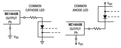
NOTE: Bipolar transistors may be added for gain (for  $V_{DD} \leq 10~V$  or  $I_{out} \geq 10~mA$ ).
