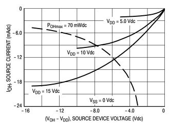
Figure 1. Typical Output Source Characteristics
