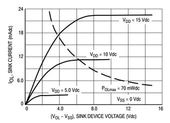
Figure 2. Typical Output Sink Characteristics
