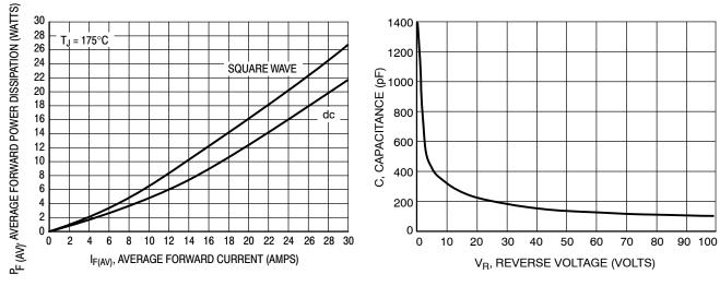
Figure 7. Forward Power Dissipation
