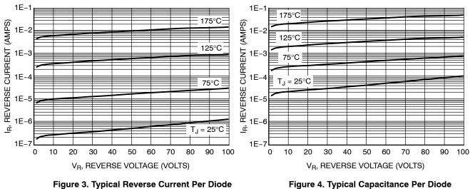
Figure 3. Typical Reverse Current Per Diode
