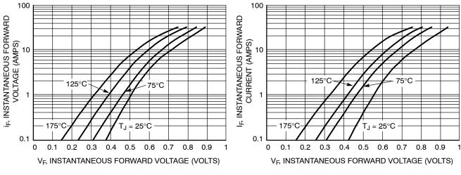
Figure 1. Typical Forward Voltage Per Diode
