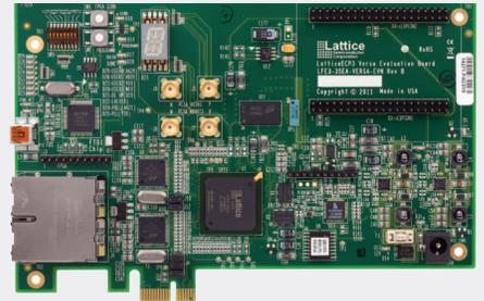
The LatticeECP3 Versa Evaluation Board is the industry's lowest cost FPGA board with PCI Express and two Gigabit Ethernet ports. It is useful for appreciating the quality of LatticeECP3 SERDES and developing a wide-range of networking and system design applications.
