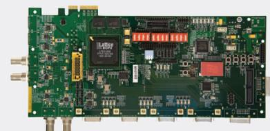
The LatticeECP3 Video Protocol Board provides a platform to evaluate the LatticeECP3 device's multi-rate 3G/HD/SDI and 7:1 LVDS capabilities. Breakout options for other display interfaces are also available.
