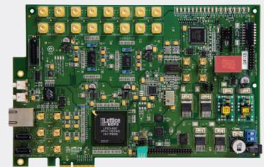
The LatticeECP3 Serial Protocol Board provides a platform to evaluate the LatticeECP3 device's multi-protocol serial protocol functionality as well as DDR2 and DDR3 memory interfaces.
