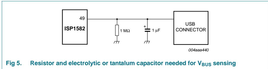
Fig 5. Resistor and electrolytic or tantalum capacitor needed for V<sub>BUS</sub> sensing
