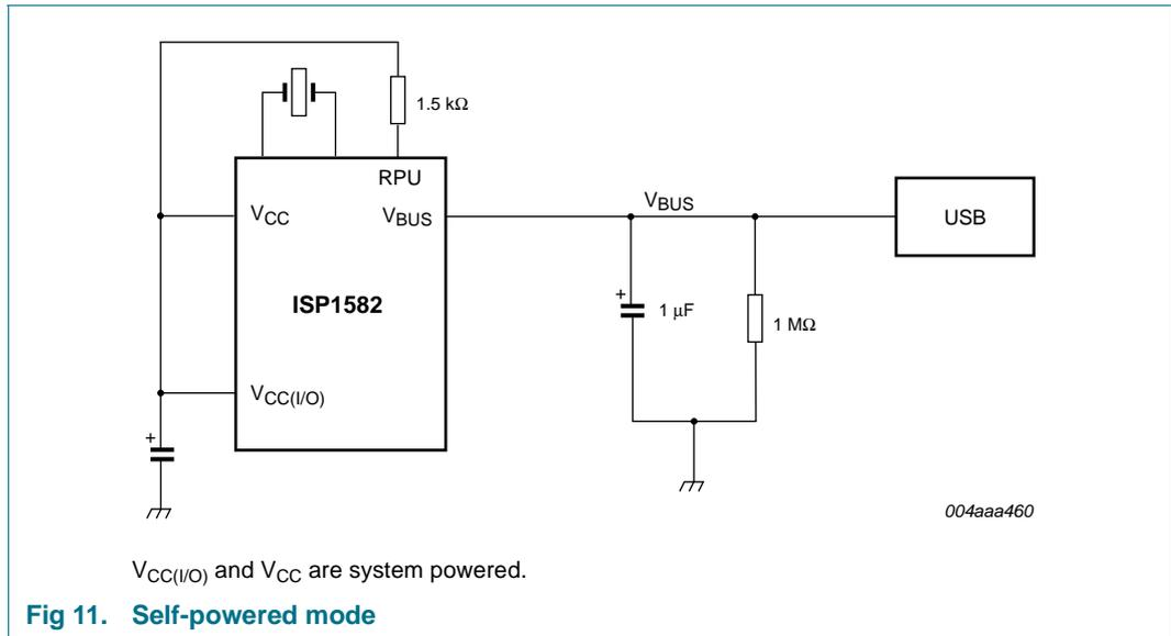
In self-powered mode, V<sub>CC</sub> and V<sub>CC(I/O)</sub> are supplied by the system. See [Figure 11](#).
