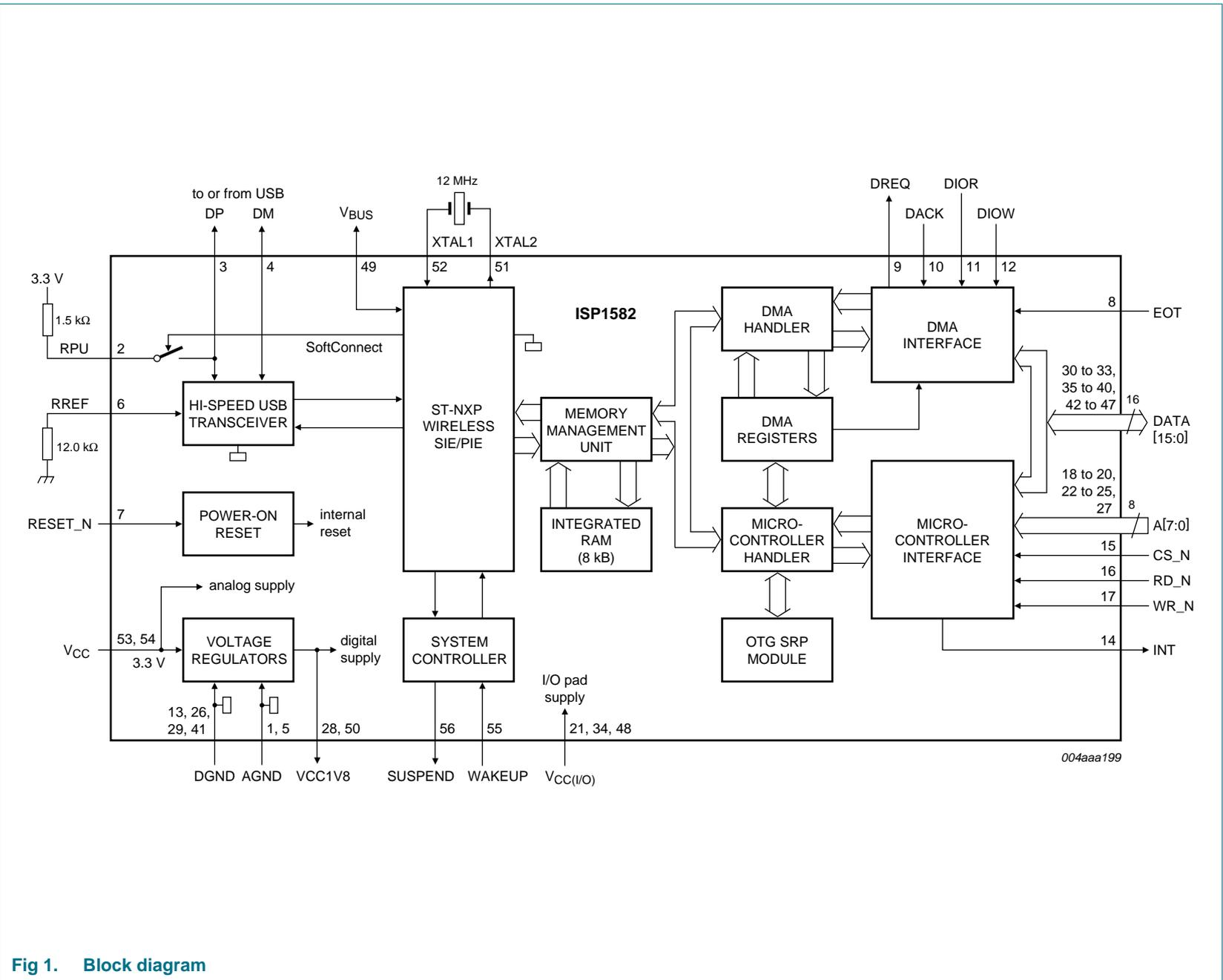
Fig 1. Block diagram
