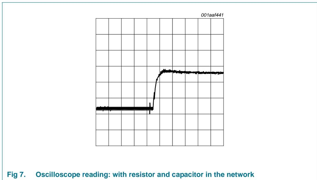
Fig 7. Oscilloscope reading: with resistor and capacitor in the network
