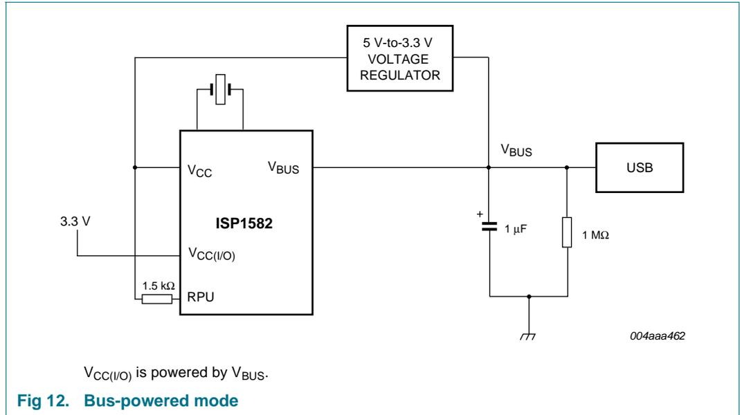
In bus-powered mode (see [Figure 12](#)), V<sub>CC</sub> and V<sub>CC(I/O)</sub> are supplied by the output of the 5 V-to-3.3 V voltage regulator. The input to the regulator is from V<sub>BUS</sub>. On plugging the USB cable, the ISP1582 goes through the power-on reset cycle. In this mode, OTG is disabled.
