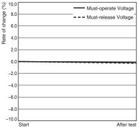
Characteristics were measured after applying vibration at a frequency of 5 to 200 to 5Hz, acceleration of 44.1 m/s<sup>2</sup> to the test piece (not energized) for 2 hours each in 3 directions.
