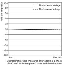
of lag chief to the test piece 3 times each in 6 directions along 3 axes. The percentage rate of change is the average value for all of the samples.
