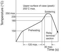
Note: The temperature profile indicates the temperature of the relay terminal section.
