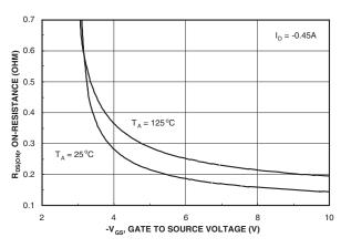
Figure 4. On-Resistance Variation with Gate-to-Source Voltage.
