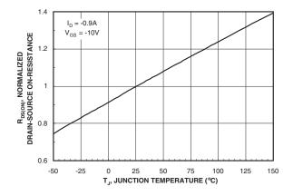
Figure 3. On-Resistance Variation with Temperature.
