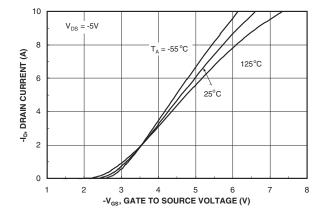
Figure 5. Transfer Characteristics.
