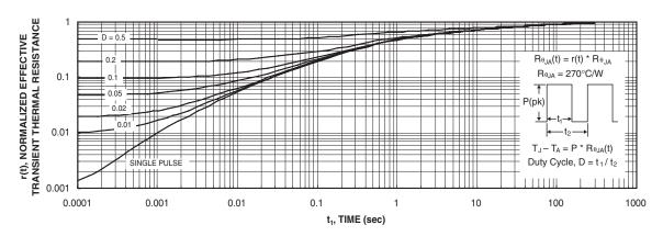
Figure 11. Transient Thermal Response Curve.
