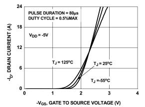
Figure 5. Transfer Characteristics
