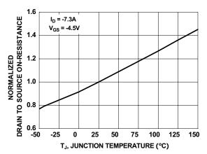
Figure 3. Normalized On-Resistance vs Junction Temperature
