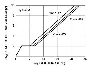
Figure 7. Gate Charge Characteristics
