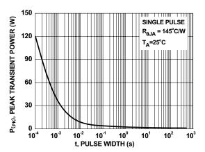
Figure 11. Single Pulse Maximum Power Dissipation
