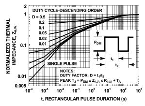
Figure 12. Transient Thermal Response Curve
