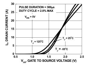
Figure 5. Transfer Characteristics
