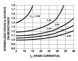
Figure 2. On-Resistance vs Drain Current and Gate Voltage
