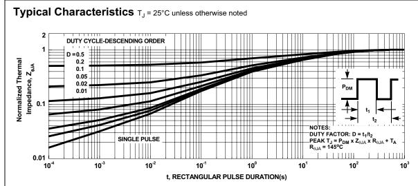
Figure 12. Transient Thermal Response Curve
