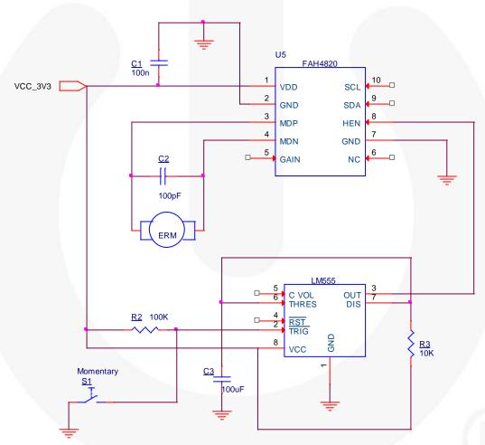
Figure 9. 555 Timer Control of Single Vibration from ERM
