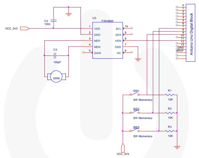
Figure 10. Arduino Uno Control HEN Pin
