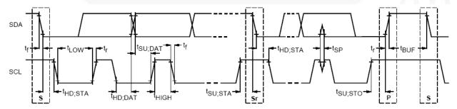
Figure 4. Definition of Timing for Full-Speed Mode Devices on the I<sup>2</sup>C Bus
