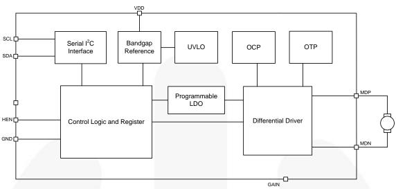
Figure 1. Block Diagram
