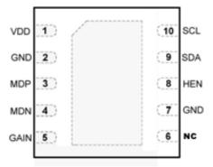
Figure 2. Pin Assignments
