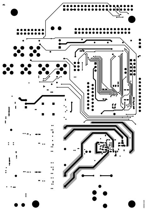
Figure 19. EVAL-AD7760/AD7762/AD7763EDZ Solder Side Layer 4 Artwork
