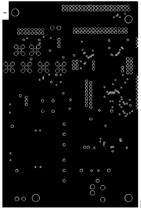
Figure 17. EVAL-AD7760/AD7762/AD7763EDZ Ground Plane Layer 2 Artwork
