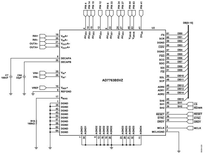
Figure 10. AD7763 Pinout for Use with EVAL-AD7760/AD7762/AD7763EDZ Schematic
