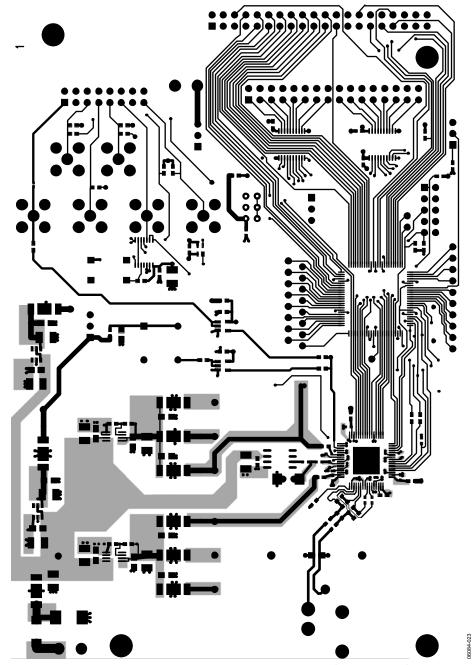
Figure 16. EVAL-AD7760/AD7762/AD7763EDZ Component Side Layer 1 Artwork
