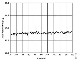
Figure 10. RTD (Platinum 100  $\Omega$ ) Sensor Input Signal Plot
