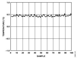
Figure 11. Fixed 100  $\Omega$  ± 1% Resistor as the Secondary Input Signal Plot
