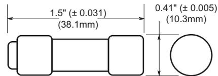
**Description:** Advanced protection Class CC current-limiting, time-delay fuses.
