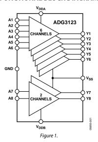
The ADG3123 is guaranteed to operate over the -40°C to +85°C temperature range and is available in a compact, 20-lead TSSOP, Pb-free package.
