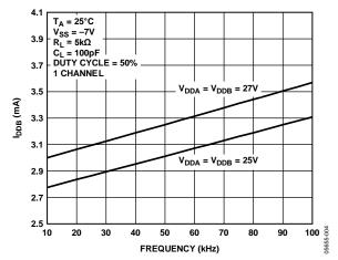
Figure 4. Supply Current (IDDB) vs. Frequency
