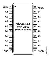
Figure 3. Pin Configuration
