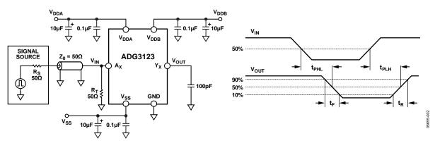
Figure 2. Switching Characteristics Test Circuit
