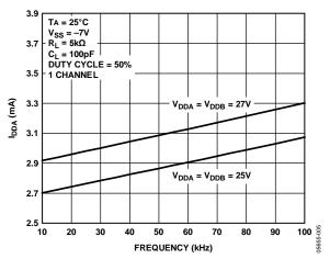
Figure 5. Supply Current (IDDA) vs. Frequency
