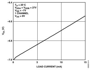
Figure 16. Output Voltage ( $V_{OL}$ ) vs. Load Current
