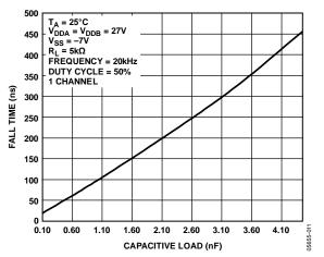
Figure 11. Fall Time vs. Capacitive Load
