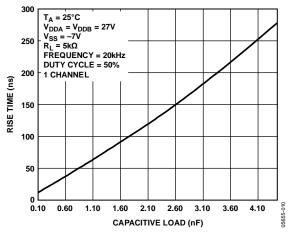
Figure 10. Rise Time vs. Capacitive Load
