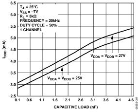
Figure 7. Supply Current (IDDB) vs. Capacitive Load
