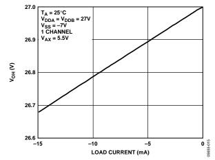
Figure 17. Output Voltage (V<sub>OH</sub>) vs. Load Current
