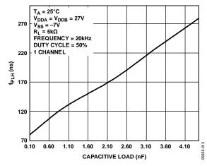
Figure 13. Propagation Delay ( $t_{PHL}$ ) vs. Capacitive Load
