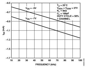
Figure 6. Supply Current (Iss) vs. Frequency
