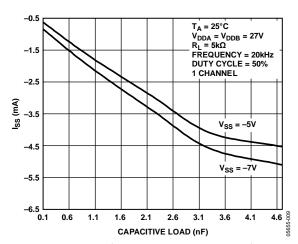
Figure 9. Supply Current (Iss) vs. Capacitive Load
