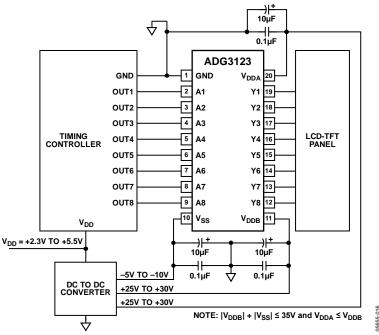
Figure 18. Typical Application Circuit
