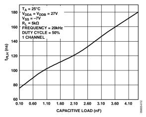
Figure 12. Propagation Delay (tplh) vs. Capacitive Load
