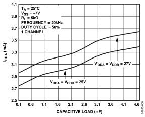
Figure 8. Supply Current (IDDA) vs. Capacitive Load
