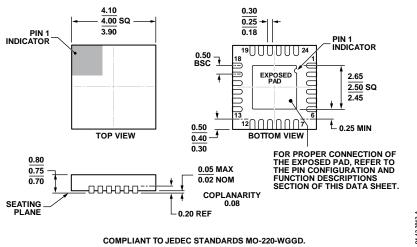
Figure 48. 24-Lead Lead Frame Chip Scale Package [LFCSP\_WQ] 4 mm × 4 mm Body, Very Very Thin Quad (CP-24-7) Dimensions shown in millimeters
