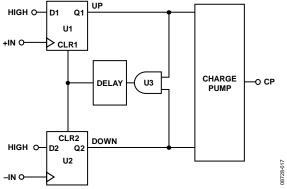
Figure 19. PFD Simplified Schematic
