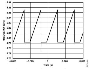
Figure 9. Delay Between Ramps for Sawtooth Waveform, PFD = 32 MHz, INT = 181, FRAC = 0, DEV Offset = 4, DEV Word = 20972, Step Word = 200, CLK<sub>2</sub> Divider = 10, CLK<sub>1</sub> Divider = 125, DEL Start Word = 1025
