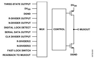
Figure 20. MUXOUT Schematic
