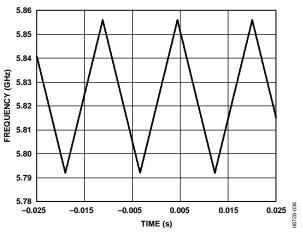
Figure 7. Triangular Waveform, PFD = 32 MHz, INT = 181, FRAC = 0, DEV Offset = 4, DEV Word = 20972, Step Word = 200, CLK<sub>2</sub> Divider = 10, CLK<sub>1</sub> Divider = 125
