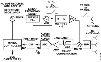
Figure 47. FMCW Radar with ADF4158
