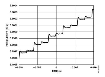
Figure 12. FSK Superimposed on Rising Edge of Triangular Waveform; Ramp Settings: PFD = 32 MHz, INT = 181, FRAC = 0, DEV Offset = 4, DEV Word = 20972, Step Word = 200, CLK DIV = 10, CLK<sub>1</sub> Divider = 125; FSK Settings: DEV Offset = 3, DEV Word = 4194
