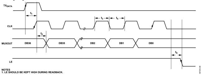
Figure 3. Read Timing Diagram
