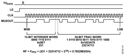
Figure 43. Reading Back Single Bits to Determine the Output Frequency at the Moment of Interrupt
