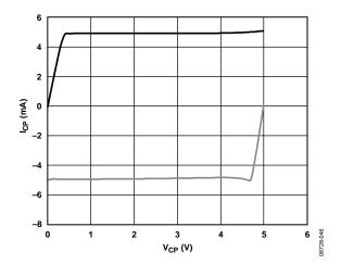
Figure 15. Charge Pump Output Characteristics
