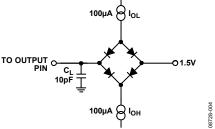
Figure 4. Load Circuit for MUXOUT Timing, C = 10 pF
