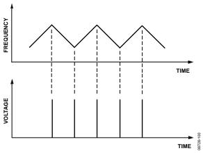
Figure 41. Ramp Complete Signal on Muxout
