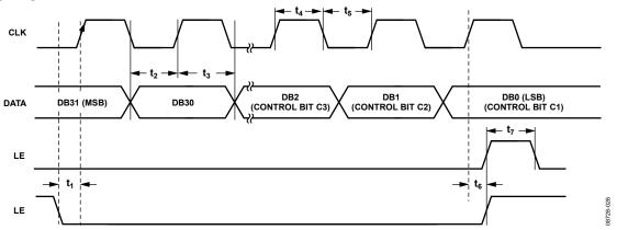
Figure 2. Write Timing Diagram
