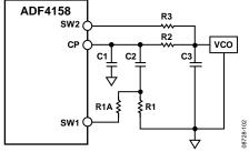
Figure 46. Fast-Lock Loop Filter Topology—Topology 2
