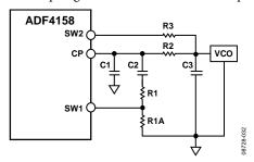
Figure 45. Fast-Lock Loop Filter Topology—Topology 1
