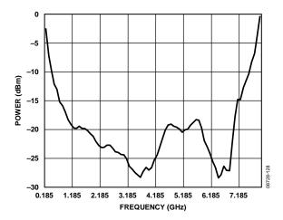
Figure 14. RF<sub>IN</sub> Sensitivity-Average Over Temperature and V<sub>DD</sub>
