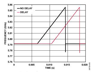
Figure 10. Delayed Start of Triangular Burst, PFD = 32 MHz, INT = 181, FRAC = 0, DEV Offset = 4, DEV Word = 20972, Step Word = 200, CLK₂ Divider = 10, CLK₁ Divider = 125, DEL Start Word = 1000
