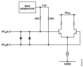
Figure 17. RF Input Stage
