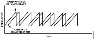
Figure 38. Delayed Start of Sawtooth Ramp
