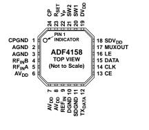
NOTES  $^{00}_{\rm L}^{\rm NOTES}$  1. THE LFCSP HAS AN EXPOSED PADDLE THAT MUST BE CONNECTED TO GND.
