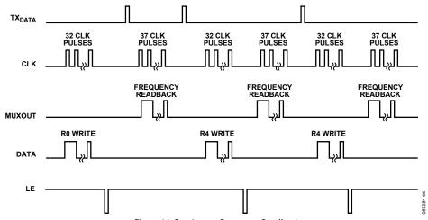
Figure 44. Continuous Frequency Readback
