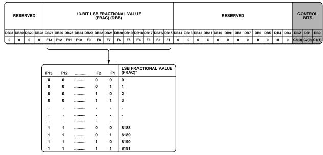
\*THE FRAC VALUE IS MADE UP OF THE 12-BIT MSB STORED IN REGISTER R0, AND THE 13-BIT LSB REGISTER STORED IN REGISTER R1. FRAC VALUE = 13-BIT LSB + 12-BIT MSB  $\times$   $2^{13}.$
