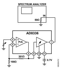
Figure 72. Input-Referred Noise vs. Source Resistance
