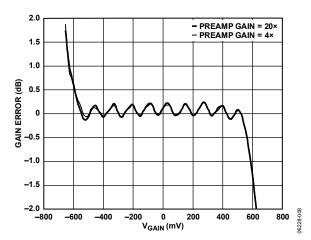
Figure 8. Gain Error vs.  $V_{GAIN}$  for Preamp Gains of 4× and 20× (See Figure 56)
