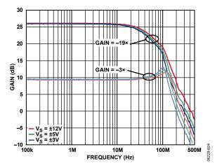
Figure 24. Preamp Frequency Response for Three Values of Supply Voltage ( $V_s$ )
