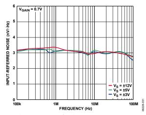
Figure 31. Short-Circuit Input-Referred Noise vs. Frequency at Maximum Gain for Three Values of Supply Voltage (Vs)
