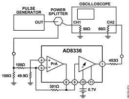
Figure 70. Pulse Response, Inverting Gain
