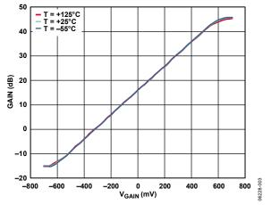
Figure 3. Gain vs.  $V_{GAIN}$  for Three Values of Temperature (T) (See Figure 56)
