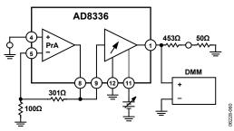
Figure 60. Offset Voltage
