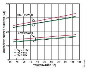
Figure 55. I<sub>Q</sub> vs. Temperature for Three Values of Supply Voltage and High and Low Power (See Figure 68)
