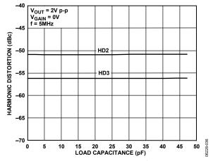
Figure 36. Harmonic Distortion vs. Load Capacitance (See Figure 64)
