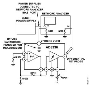
Figure 71. Power Supply Rejection Ratio
