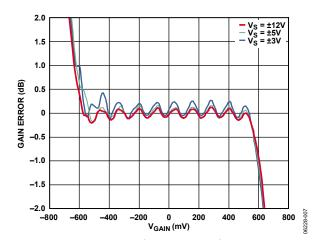
Figure 7. Gain Error vs. V<sub>GAIN</sub> for Three Values of Supply Voltage (V<sub>s</sub>) (See Figure 56)
