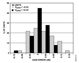
Figure 12. Gain Error Histogram
