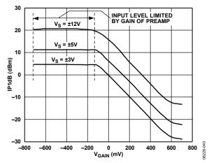
Figure 43. Input P1dB (IP1dB) vs. V<sub>GAIN</sub> at Three Power Supply Values (V<sub>s</sub>) (see Figure 74 and Figure 75)
