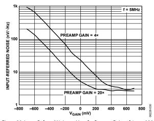
Figure 30. Input-Referred Noise vs.  $V_{GAIN}$  for Preamp Gains of 4× and 20× (See Figure 62)
