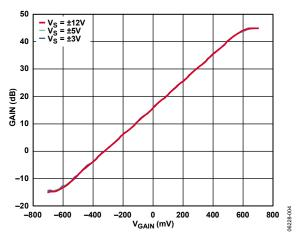
Figure 4. Gain vs. V<sub>GAIN</sub> for Three Values of Supply Voltage (V<sub>s</sub>) (See Figure 56)
