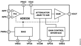
Figure 79. Application Block Diagram
