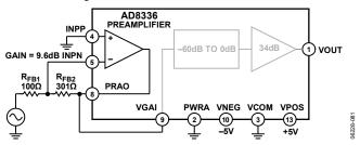
Figure 81. Circuit Configuration for Inverting Gain
