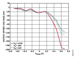
Figure 15. Output Offset Voltage vs. V<sub>GAIN</sub> for Three Values of Supply Voltage (Vs)
