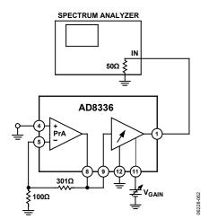
Figure 62. Input-Referred Noise and Output-Referred Noise
