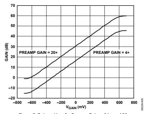
Figure 5. Gain vs.  $V_{GAIN}$  for Preamp Gains of 4× and 20× (See Figure 56)
