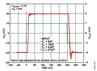
Figure 50. Large-Signal Pulse Response for Various Values of Load Capacitance Using ±5 V Power Supplies (See Figure 65)
