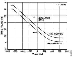
Figure 34. Noise Figure vs. V<sub>GAIN</sub> (See Figure 63)
