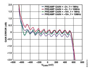
Figure 10. Gain Error vs. V<sub>GAIN</sub> at 1 MHz and 10 MHz and for Inverting Preamp Gains of -3× and -19× (See Figure 56)
