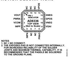
Figure 2. Pin Configuration
