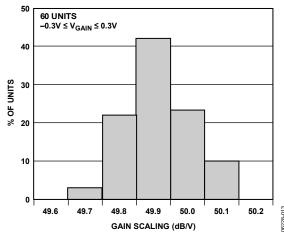
Figure 13. Gain Scaling Factor Histogram
