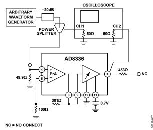
Figure 67. VGA Overdrive Recovery
