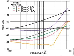
Figure 54. PSRR vs. Frequency for Three Values of V<sub>GAIN</sub> (See Figure 71)
