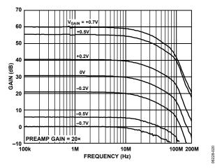
Figure 20. Frequency Response for Various Values of V<sub>GAIN</sub>
