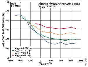
Figure 38. Second Harmonic Distortion vs. V<sub>GAIN</sub> for Four Values of Output Voltage (V<sub>OUT</sub>)
