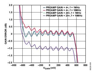
Figure 9. Gain Error vs. V<sub>GAIN</sub> at 1 MHz and 10 MHz and for Preamp Gains of 4× and 20× (See Figure 56)
