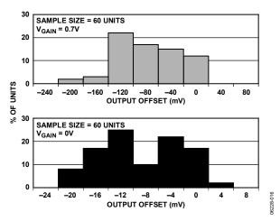
Figure 16. Output Offset Histogram
