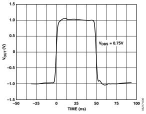
Figure 34. Full-Scale Transient Response,  $V_{\rm DBS}$  = 0.75 V, f = 1 MHz,  $V_{\rm OUT}$  = 2 V p-p
