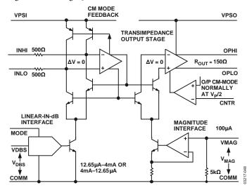
Figure 47. Schematic of Key Components
