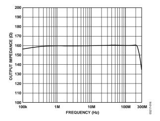
Figure 15. Output Impedance vs. Frequency
