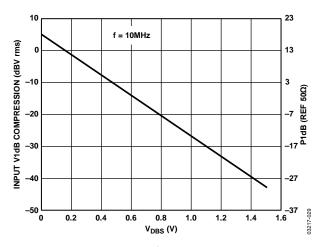
Figure 28. Input V1dB Compression vs.  $V_{DBS}$
