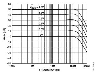
Figure 9. Frequency Response in 10 dB Steps for Various Values of  $V_{\rm DBS}$
