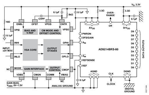
Figure 63. Driving an Analog-to-Digital Converter (Preliminary)
