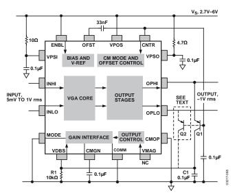
Figure 64. Simple AGC Amplifier (Preliminary)
