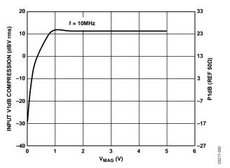
Figure 29. Output V1dB Compression vs.  $V_{MAG}$
