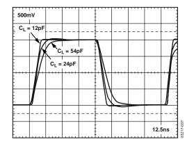
Figure 36. Transient Response vs. Various Load Capacitances,  $G=25\,dB$
