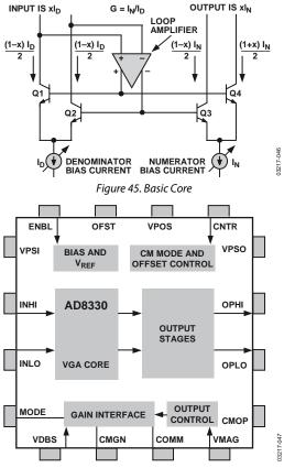
Figure 46. Block Schematic
