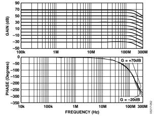
Figure 51. AC Performance over a 100 dB Gain Range Obtained by Using Two Values of V<sub>MAG</sub>
