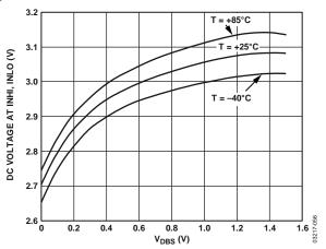
Figure 55. Common-Mode Voltage at Input Pins vs.  $V_{DBS}$  for  $V_S$  = 5 V, T =  $-40^{\circ}$ C,  $+25^{\circ}$ C, and  $+85^{\circ}$ C
