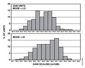
Figure 8. Gain Slope Histogram
