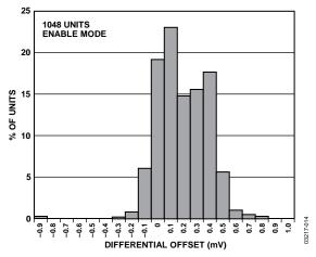
Figure 13. Differential Input Offset Histogram
