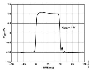
Figure 35. Full-Scale Transient Response,  $V_{DBS}$  = 1.5 V, f = 1 MHz,  $V_{OUT}$  = 2 V p-p
