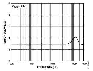
Figure 11. Group Delay vs. Frequency
