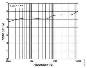
Figure 22. Input Referred Noise vs. Frequency
