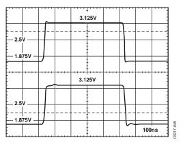
Figure 44. CNTR Transient Response, Top: Input to CNTR, Bottom:  $V_{\text{OUT}}$  Single-Ended
