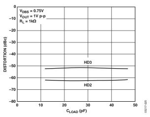
Figure 24. Harmonic Distortion vs.  $C_{LOAD}$
