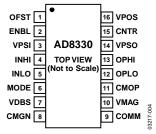
Figure 3. 16-Lead QSOP Pin Configuration
