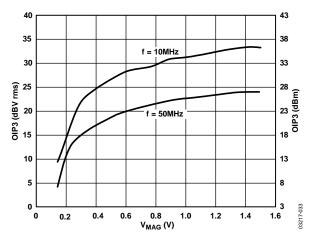
Figure 32. OIP3 vs.  $V_{MAG}$
