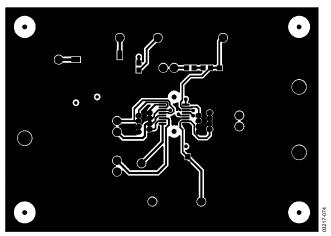
Figure 73. Component-Side Wiring
