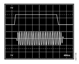
Figure 37.  $V_{DBS}$  Interface Response, Top:  $V_{DBS}$ , Bottom:  $V_{OUT}$
