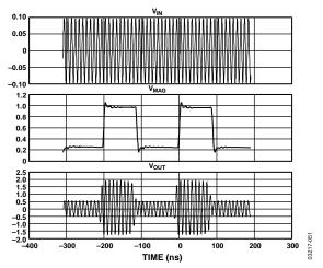
Figure 50. Using VMAG in Modulation Mode
