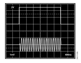
Figure 38.  $V_{MAG}$  Interface Response, Top:  $V_{MAG}$ , Bottom:  $V_{OUT}$
