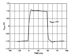
Figure 33. Full-Scale Transient Response,  $V_{DBS} = 0 V$
