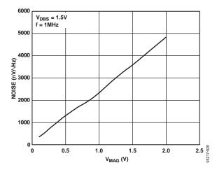
Figure 19. Output Referred Noise vs.  $V_{MAG}$
