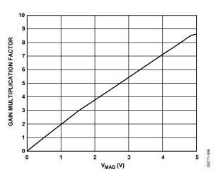
Figure 5. Linear Gain Multiplication Factor vs.  $V_{MAG}$
