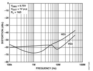
Figure 23. Harmonic Distortion vs. Frequency
