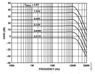
Figure 10. Frequency Response for Various Values of  $V_{\rm NAG}$ ,  $V_{\rm DBS} = 0.75~{\rm V}$
