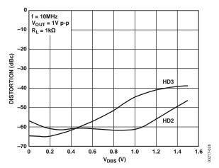
Figure 27. Harmonic Distortion vs.  $V_{\rm DBS}$
