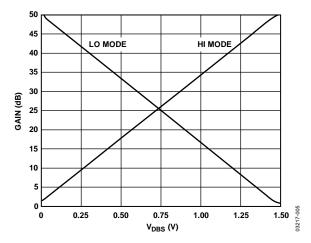
Figure 4. Gain vs. V<sub>DBS</sub>
