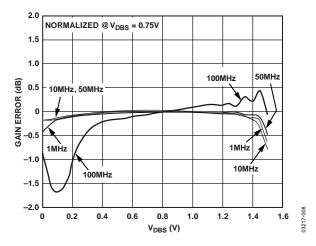
Figure 7. Gain Error vs. V<sub>DBS</sub> at Various Frequencies
