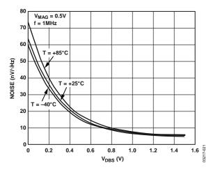
Figure 20. Input Referred Noise vs.  $V_{\rm DBS}$  for Three Temperatures
