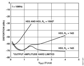
Figure 26. Harmonic Distortion vs.  $V_{OUT}$ ,  $V_{MAG} = 2.0 \text{ V}$
