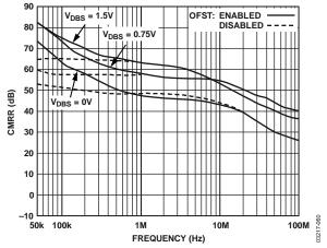
Figure 59. Input CMRR vs. Frequency for Various Values of  $V_{\rm DBS}$
