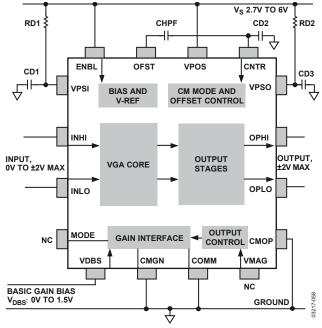
Figure 57. Power Supply Decoupling and Basic Connections
