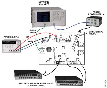
Figure 71. Typical Connections
