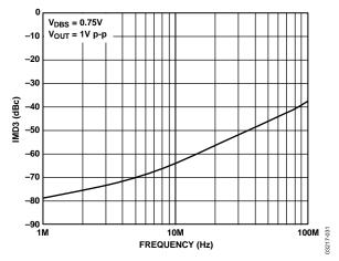
Figure 30. IMD3 Distortion vs. Frequency
