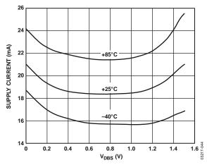
Figure 43. Supply Current vs. V<sub>DBS</sub> at Three Temperatures
