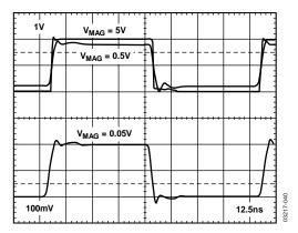
Figure 39. Transient Response vs.  $V_{\rm MAG}$
