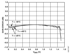
Figure 6. Gain Linearity Error Normalized at 25°C vs.  $V_{D85}$  at Three Temperatures, f = 1 MHz
