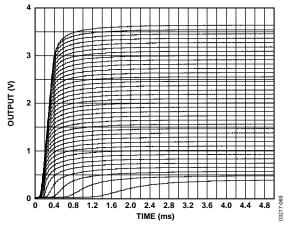
Figure 68. Time Domain Response of RMS Voltmeter (Simulation)
