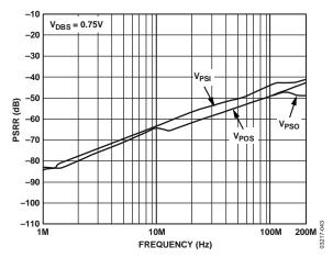
Figure 42. PSRR vs. Frequency
