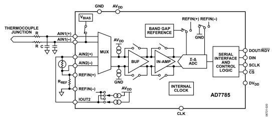
Figure 20. Thermocouple Measurement Using the AD7785
