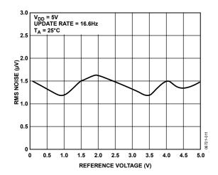
Figure 11. RMS Noise vs. Reference Voltage (Gain = 1)
