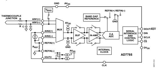
Figure 12. Basic Connection Diagram
