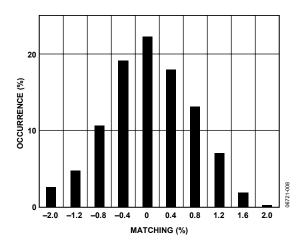
Figure 8. Excitation Current Matching (210 μA) at Ambient Temperature
