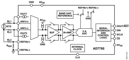
Figure 21. RTD Application Using the AD7785
