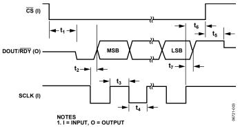
Figure 3. Read Cycle Timing Diagram
