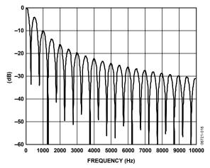
Figure 16. Filter Response at 470 Hz Update Rate
