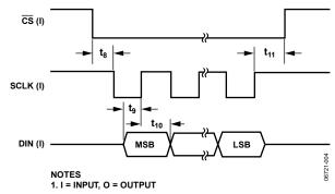
Figure 4. Write Cycle Timing Diagram
