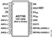
Figure 5. Pin Configuration
