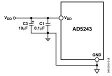
Figure 43. Power Supply Bypassing
