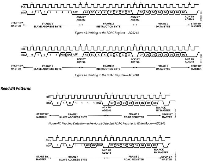
Figure 48. Reading Data from a Previously Selected RDAC Register in Write Mode—AD5248
