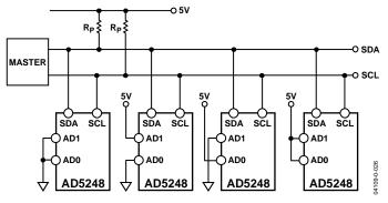
Figure 49. Multiple AD5248 Devices on One I<sup>2</sup>C Bus
