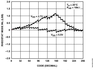
Figure 6. R-INL vs. Code vs. Supply Voltages
