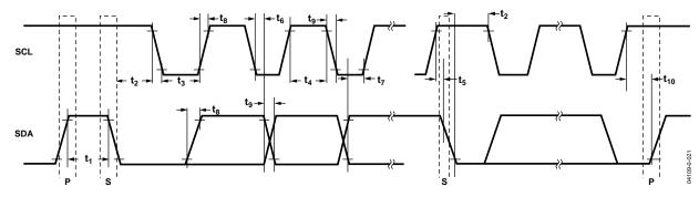
Figure 3. I<sup>2</sup>C Interface Detailed Timing Diagram
