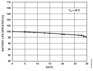
Figure 44. Battery Operating Life Depletion
