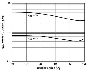
Figure 16. Supply Current vs. Temperature
