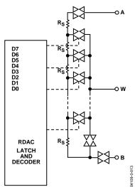
Figure 38. AD5243 Equivalent RDAC Circuit
