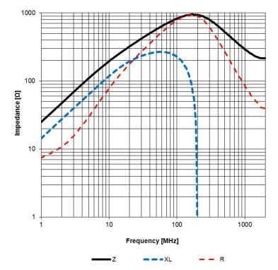
Test Equipment: E4991A or equivalent
