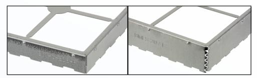
SEdB  $\approx$  100 -20 log( wfMH) + 20log[1+ln(w/h)] + 30 (t/w) | w<  $\lambda$ /2 where w is length of slot and w>h and w>>t;  $\lambda$  is wavelength in meter; fMH is frequency in MHz.
