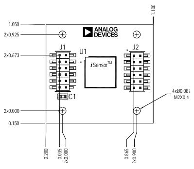
Figure 3. ADIS16XXX/PCB Mechanical Drawing
