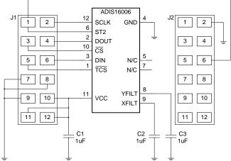
Figure 1 - ADIS16006/PCBZ Schematic
