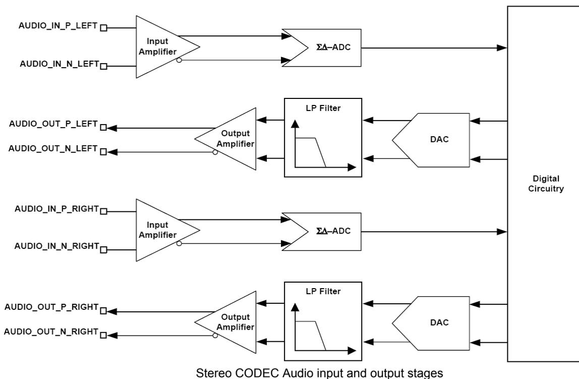
The stereo audio CODEC uses a fully differential architecture in the analogue signal path, which results in low noise sensitivity and good power supply rejection while effectively doubling the signal amplitude.
