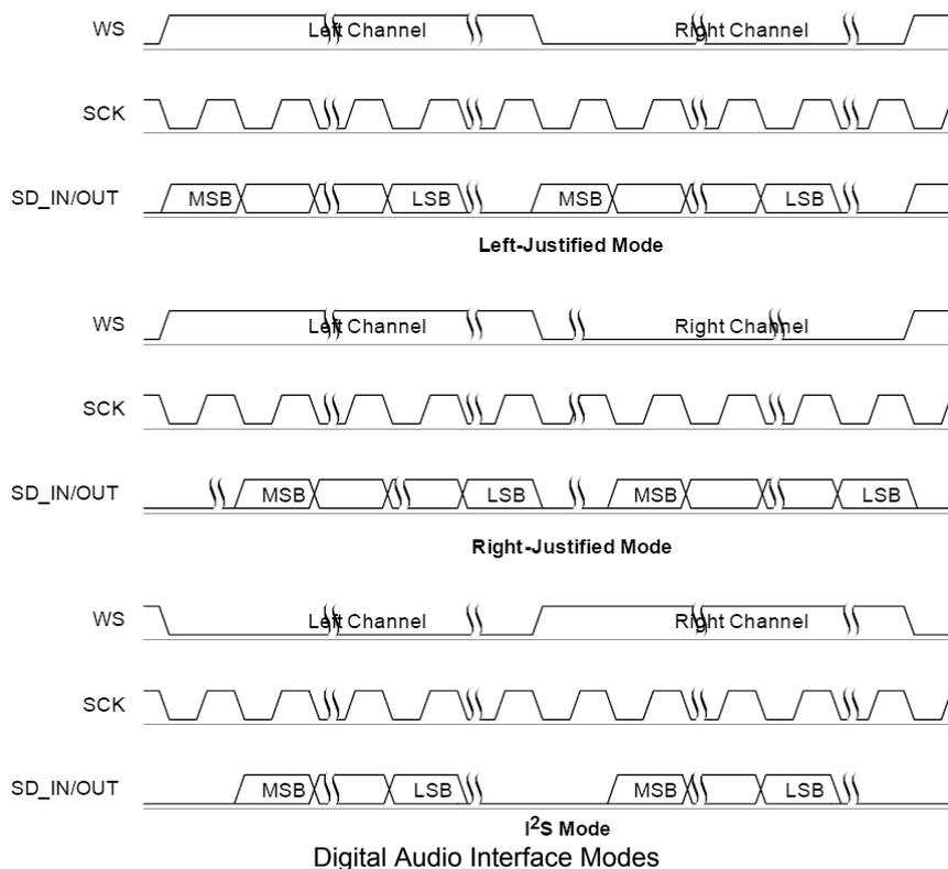
The internal representation of audio samples within F2M03MLA is 16-bit and data on SD\_OUT is limited to 16-bit per channel. On SD\_IN, if more than 16-bit per channel is present will round considering the 17<sup>th</sup> bit.
