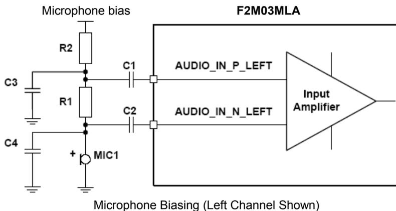
The input impedance at AUDIO\_IN\_N\_LEFT, AUDIO\_IN\_P\_LEFT, AUDIO\_IN\_N\_RIGHT and AUDIO\_IN\_P\_RIGHT is typically  $20\text{k}\Omega$ . C1 and C2 should be  $47\text{nF}$ . R1 sets the microphone load impedance and is normally in a range of 1 to  $2\text{k}\Omega$ . R2, C3 and C4 improve the supply rejection by decoupling supply noise from the microphone. Values should be selected as required in the specification. R2 may be connected to a convenient supply (typically VDD).
