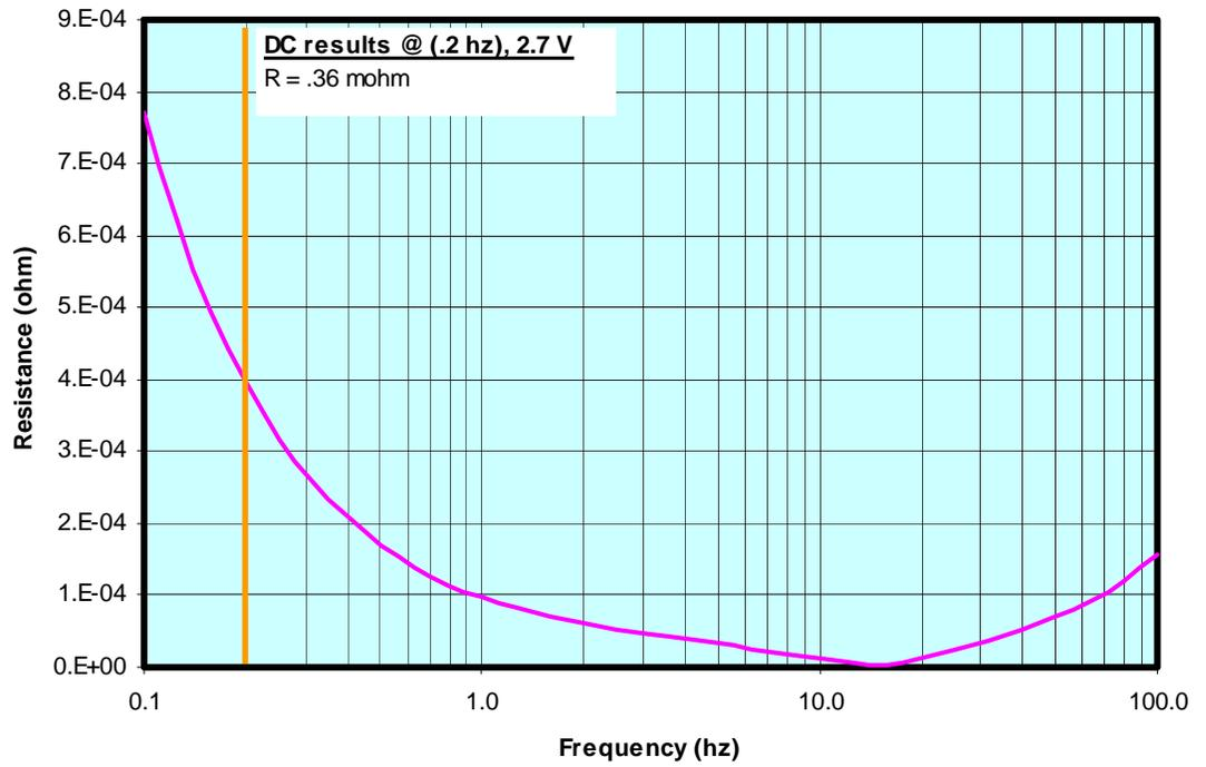
Figure 15: BCAP2600 Resistance Frequency Response
