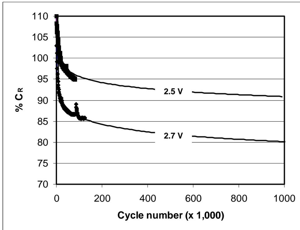
Figure 6: Capacitance change vs. Continuous cycling
