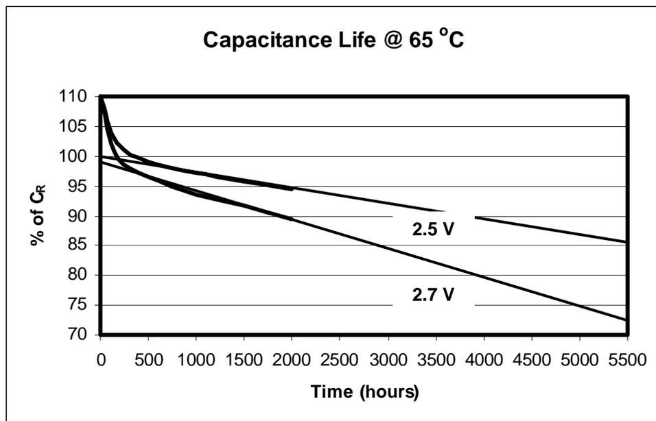
Figure 4: MC Cell Capacitance degradation at 2.7 V and 2.5 V at 65oC
