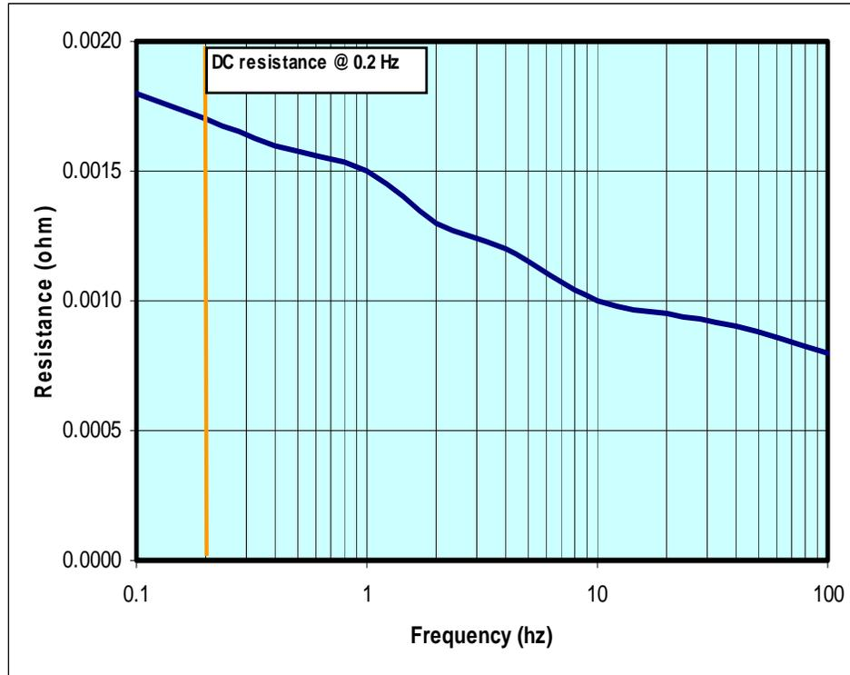
Figure 13: BCAP0350 Resistance Frequency Response
