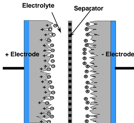
Figure 1: Ultracapacitor charge separation
