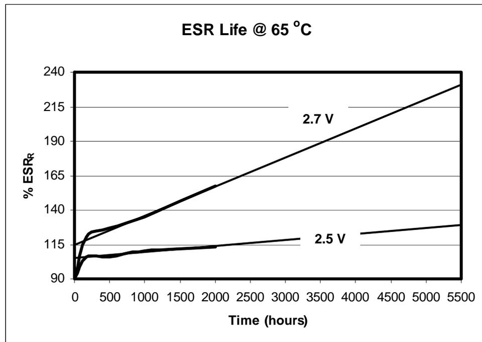
Figure 5: MC Cell Resistance degradation at 2.7 V and 2.5 V at 65oC
