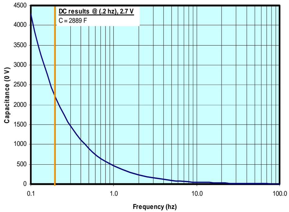
Figure 14: BCAP2600 Capacitance Frequency Response
