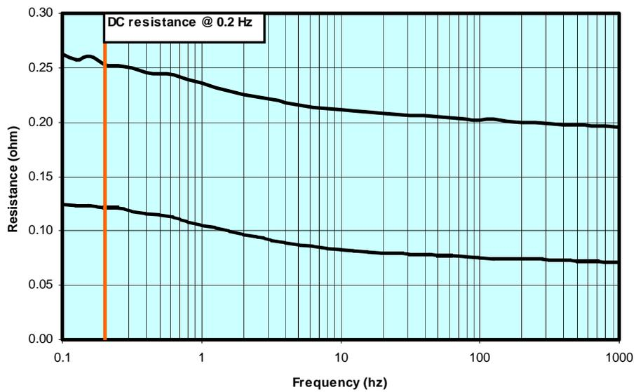
Figure 11: PC10 Resistance vs. Frequency Response, 95% Confidence
