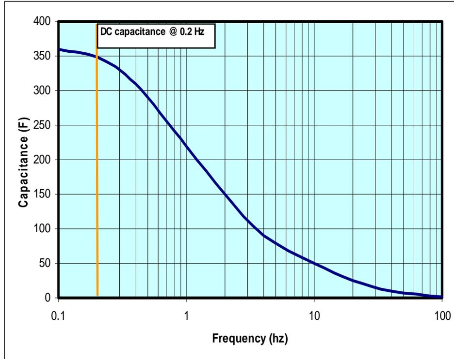
Figure 12: BCAP0350 Capacitance Frequency Response
