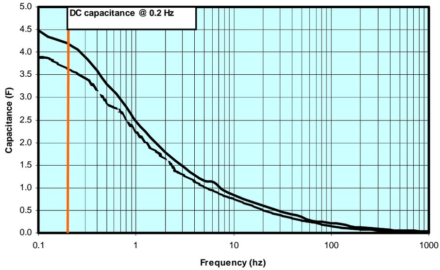
Figure 8: PC5 Capacitance vs. Frequency Response, 95% Confidence
